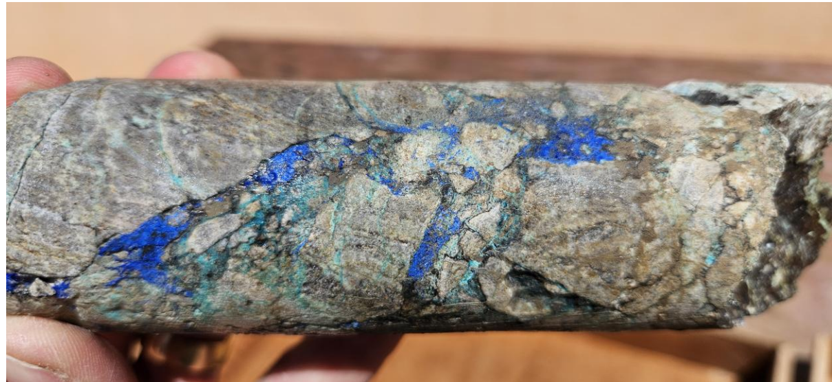
Core sample from DDH M-2 at the core interval of 284.45m showing fracture-controlled azurite (blue) and malachite (green) copper mineralization.
