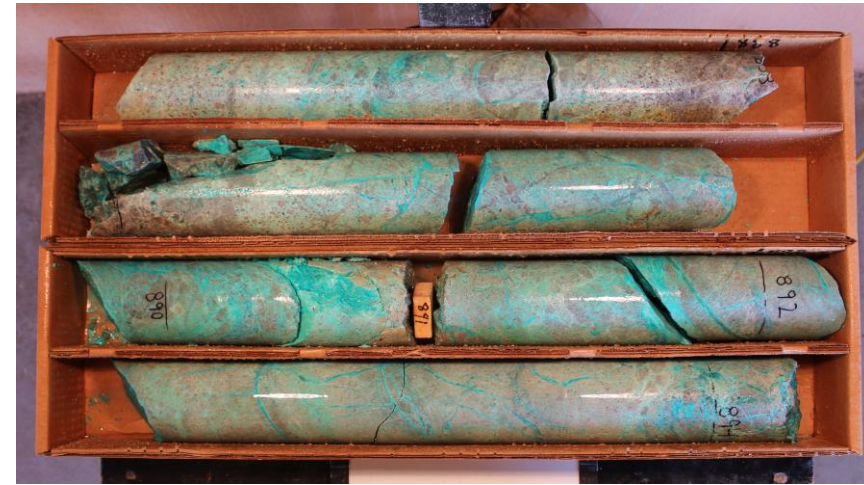
DDH VD14-06 3.29% AsCu 270.05m – 272.58m Malachite and chrysocolla in Pinal Schist
