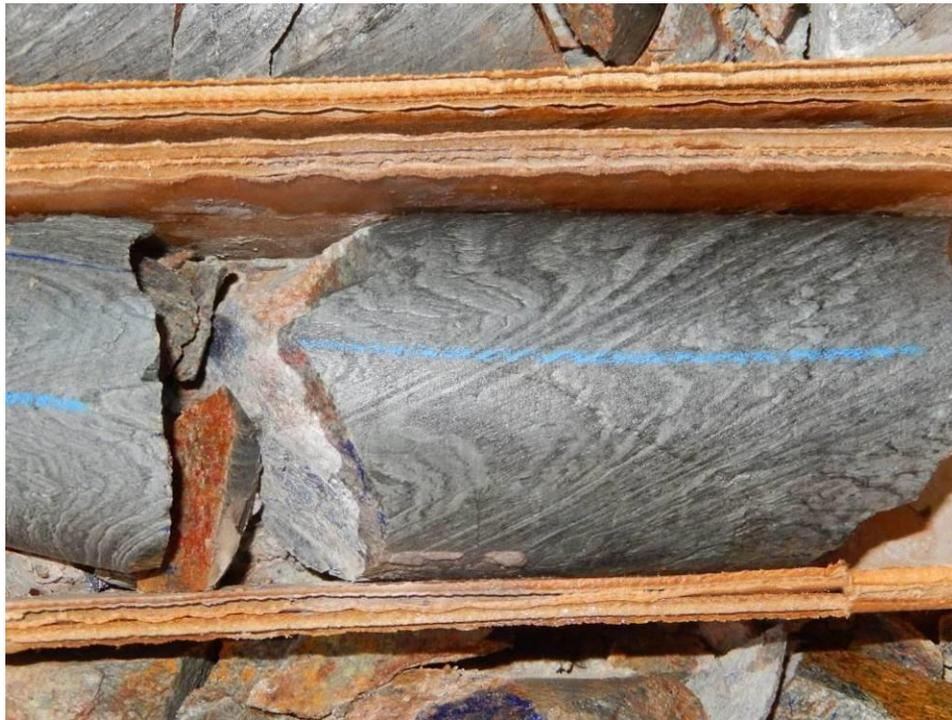
**Plate 7-1**      **Chevron-folded Pinal Schist, Drillhole VD-14-05 at 439.7m**
