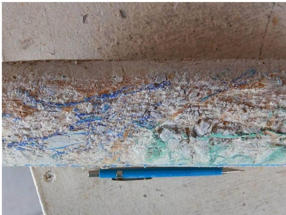
**Plate 7-2**      **Brecciated Pinal Schist re-cemented in part by azurite and malachite, Drillhole VD-14-04 at 473.3m [the linear alignment of the mineralized structure suggests mineralized fracture]**
