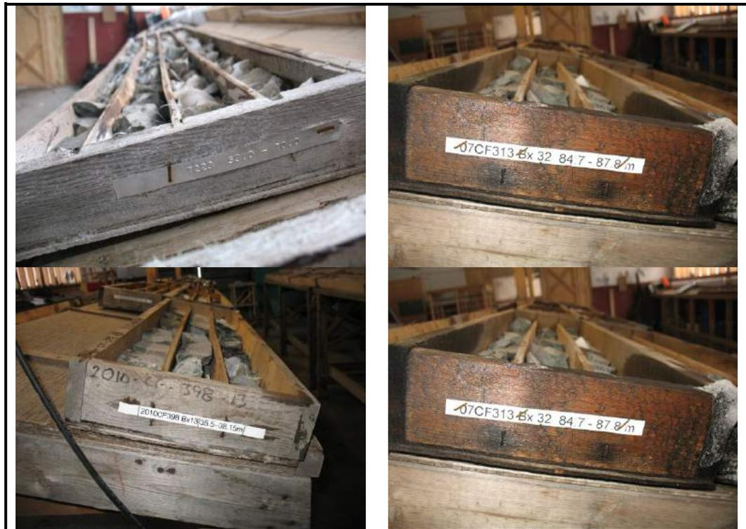
Note: Poor core recovery also shown (broken ground)
