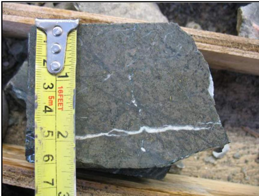
**Figure 12.17 8CF-327 Sample 147199 – Disseminated Sulphides (Chalcopyrite + Pyrite)**
