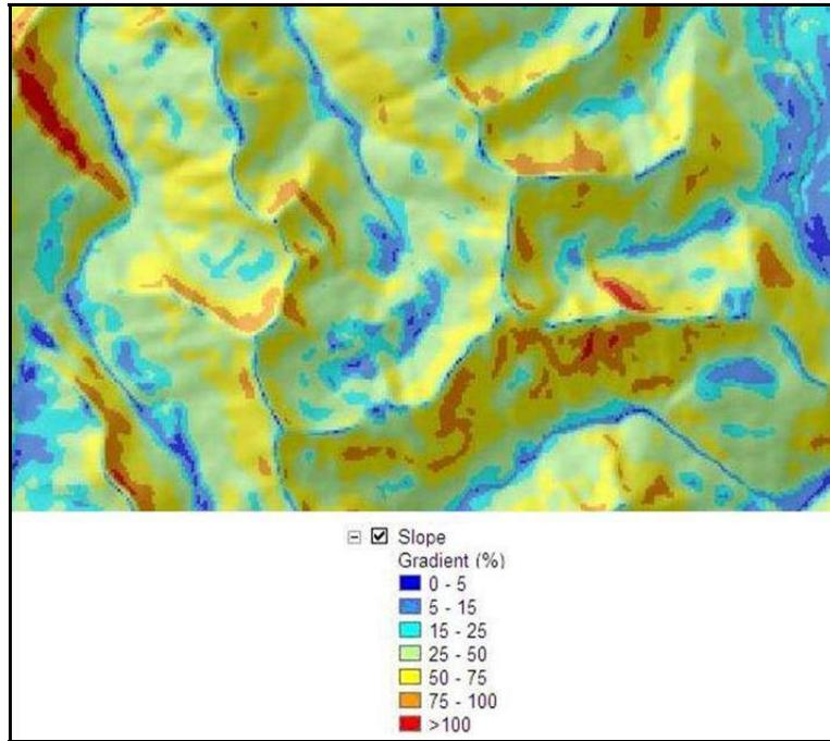
Plate 4.4-3. Example of the Slope concept.
