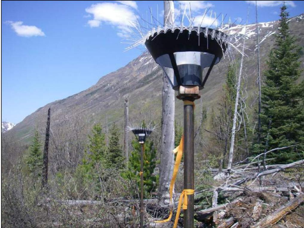
*Plate 2.6-1. Baseline dustfall monitoring station FD3, including two individual dustfall canisters (white) surrounded by a wind screen (black) and bird spikes (metal). Two containers are needed to collect a sufficient volume of sample for the list of parameters.*
