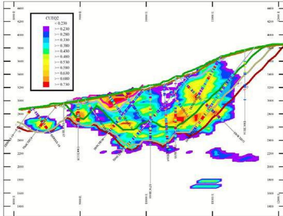
Cross Section at 24000N Showing Optimized Pit Outlines and Grade Model with Net Copper Equivalent
