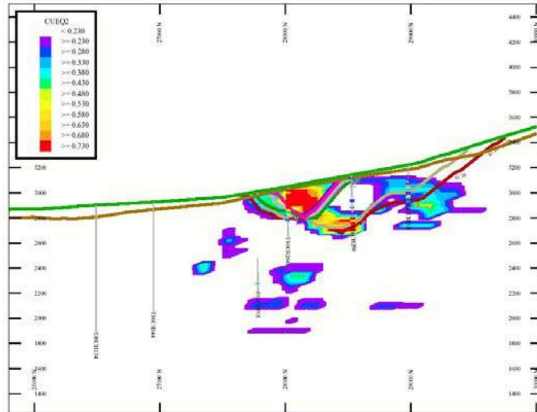
Long Section at 7300E Showing Optimized Pit Outlines and Grade Model with Net Copper Equivalent
