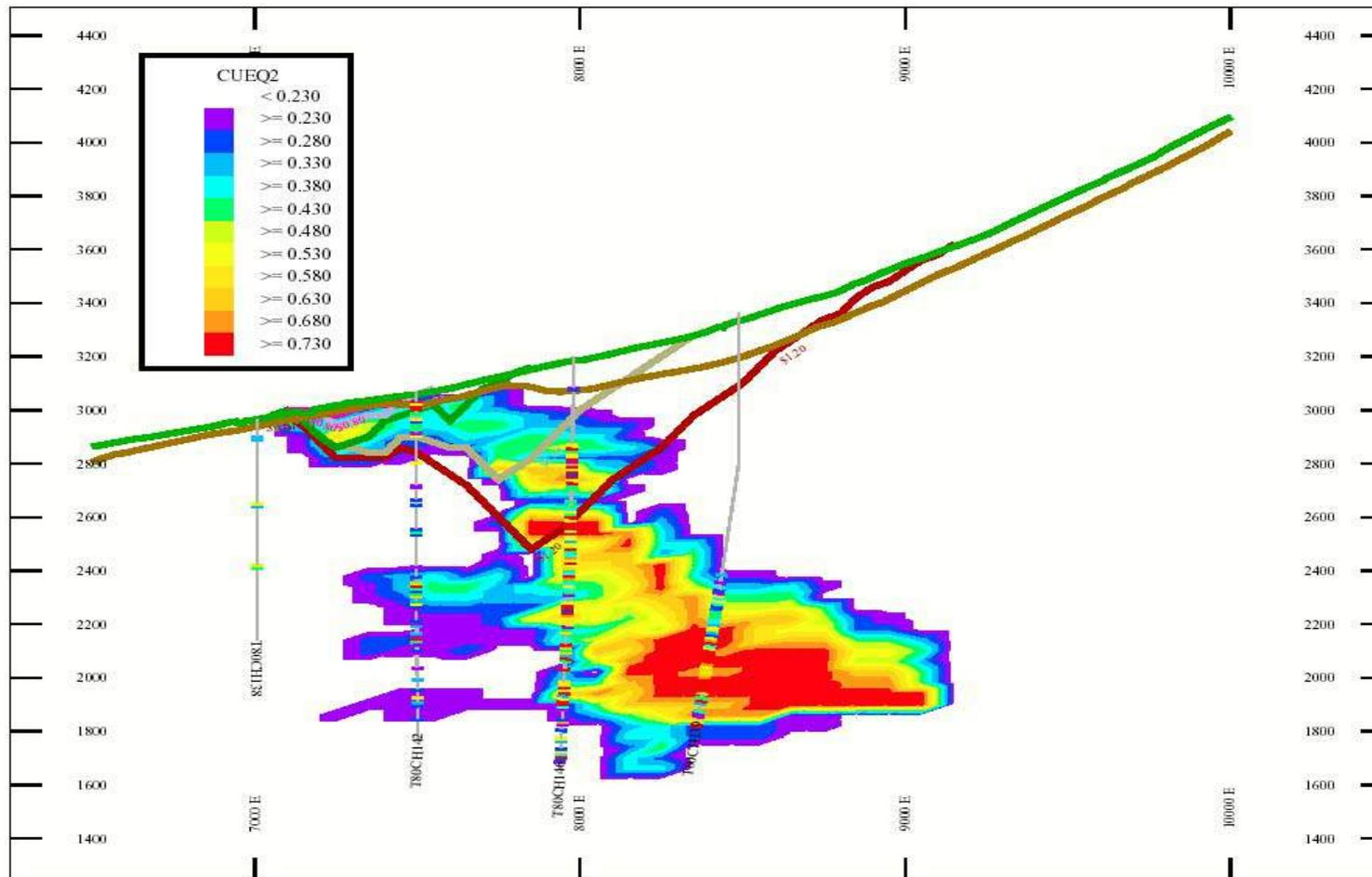
Cross Section at 27900N Showing Optimized Pit Outlines and Grade Model with Net Copper Equivalent
