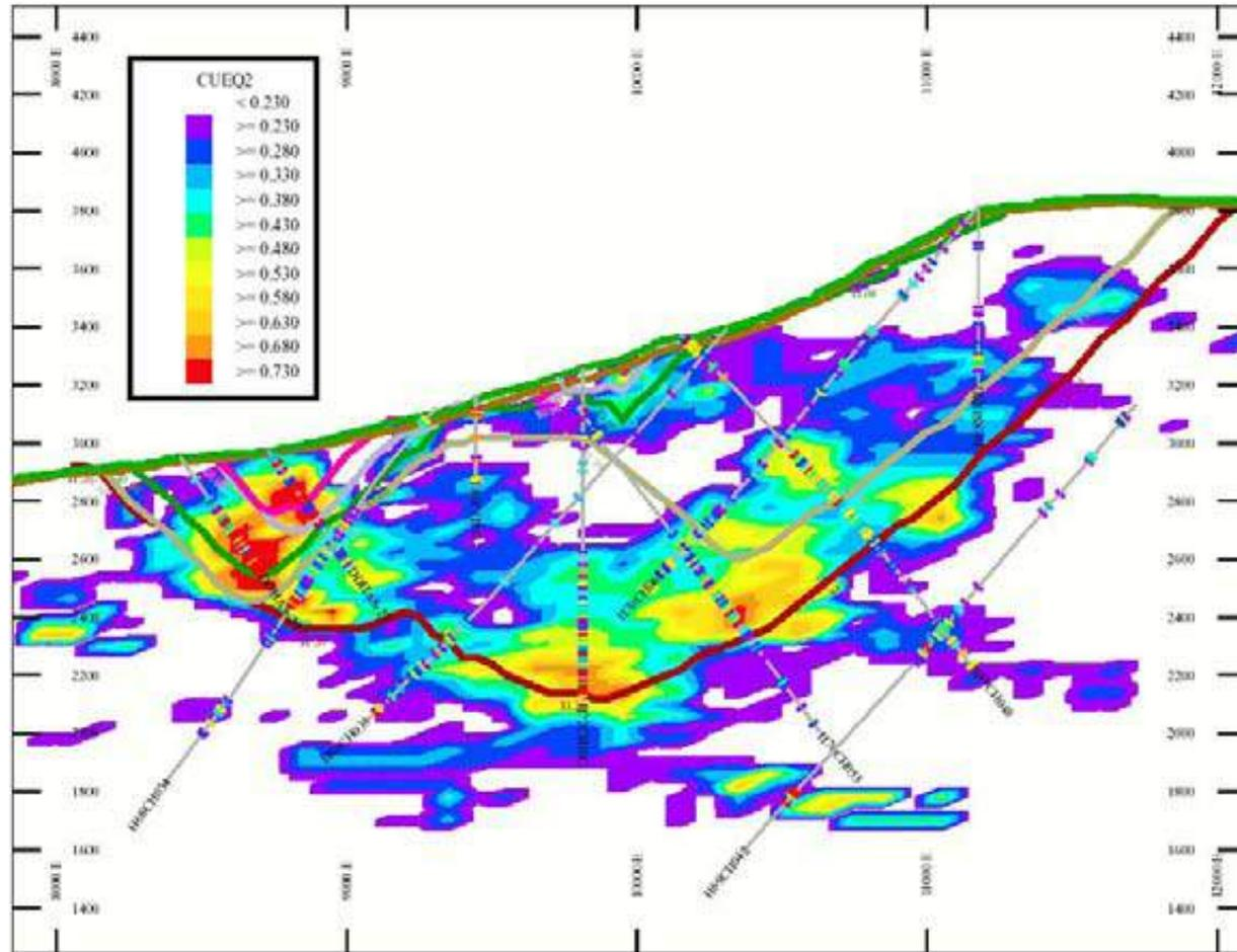
Cross Section at 24900N Showing Optimized Pit Outlines and Grade Model with Net Copper Equivalent
