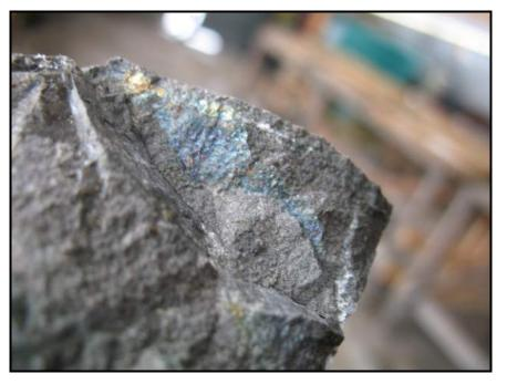
Figure 12.11 T81CH223 at 53 m – Bornite + Chalcopyrite, Core of NQ Diameter
