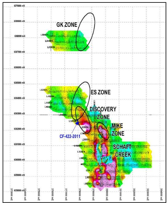
Figure 9.3Results of the Quantec Titan 24 IP and MT Survey, with<br/>Chargeability Anomalies Outlined
