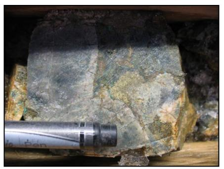
Figure 12.14 10CF-398 Sample 611051 – Malachite + Sulphides
